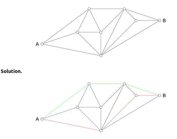
Note that there are three paths (coloured) from A to city B such that no two distinct paths share a road in common. Thus, in order to disconnect cities A and B by removing roads, at least one road must be removed from each of these three paths. Therefore, the answer is at least 3. On the other hand, removing the roads coming out of city A disconnects A from B, so removing three roads can disconnect cities A and B.
